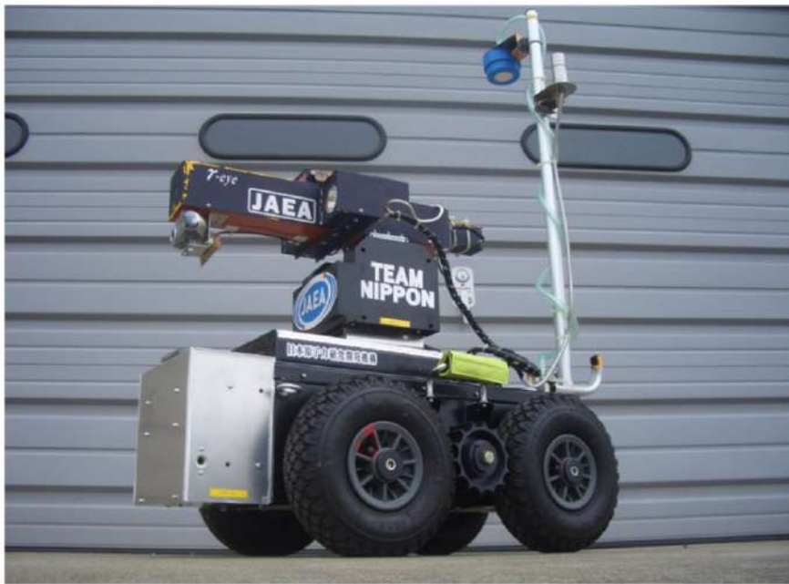
Fig. 6 JAEA-3 robot equipped with gamma imaging and measurement device
