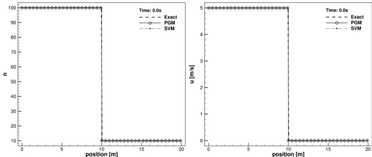
For the whole domain  $\Theta_{xx}$  is equal to  $1.0 \text{ m}^2/\text{s}^2$ ,  $\Psi_{xd}$  is equal to  $0 \text{ m/s}$ ,  $\mu$  is equal to  $\ln(28 \times 10^{-6})$  and  $\Psi_{dd}$  is equal to  $0.25$ . A grid of 4000 cells with a CFL number of 0.5 is used for all cases.
