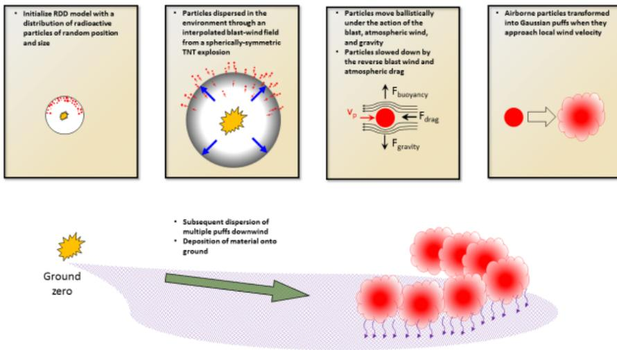
**Figure:** 1) Initialization of particles in the explosive device, 2) outward acceleration in the blast field, 3) deceleration in the atmosphere, 4) conversion to a Gaussian puff, and the subsequent dispersion and deposition onto the ground.
