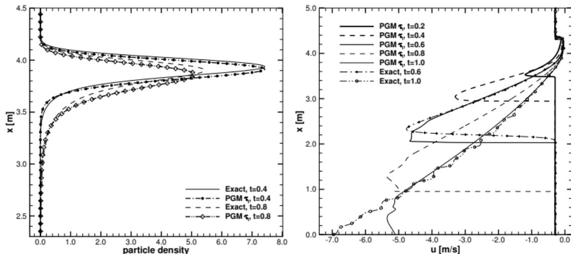
Figure: Comparison between the PGM predictions and exact solution for the particle density and velocity as a function of the vertical spatial coordinate
