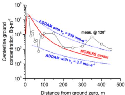
(c) Ground deposition profile along plume centreline
